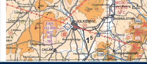
↑ (B) EXAMPLE OF MAXIMUM ELEVATION FIGURE (MEF)
