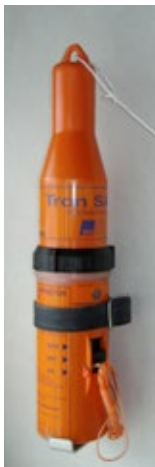
SARTs provide a homing signal on a radar screen
