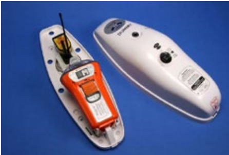
An EPIRB is a distress alerting device
