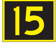
Runway Location Sign
