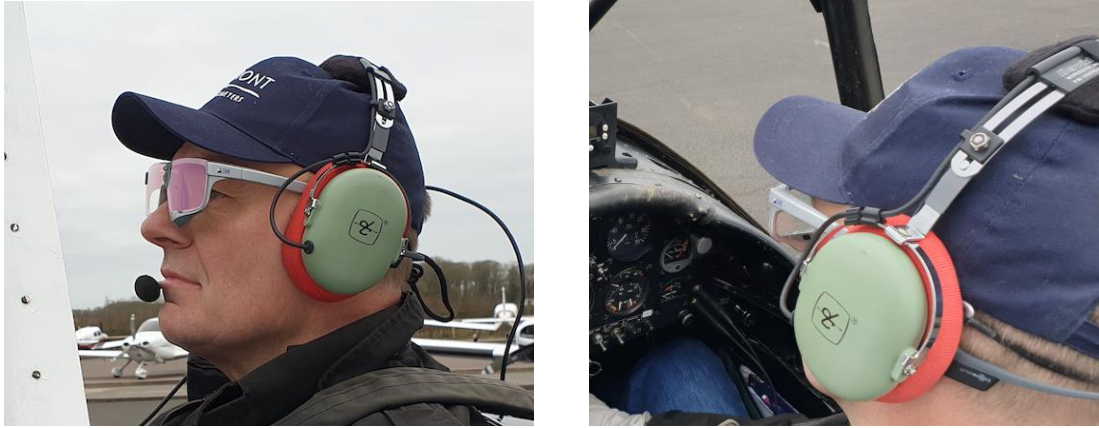
Figure 4. Pilot wearing SMI 'Natural Gaze' 60Hz eye-tracking glasses.
