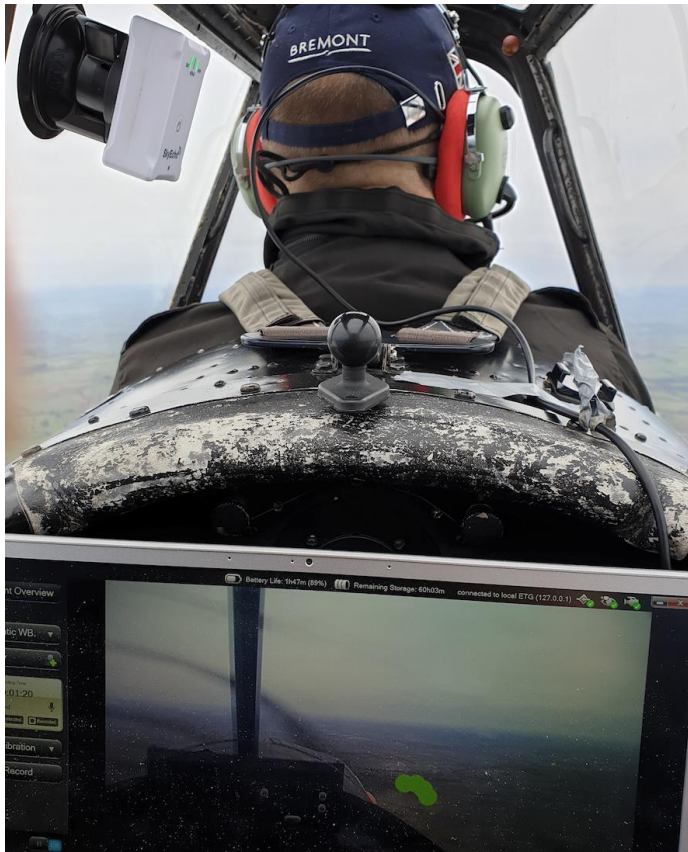
Figure 14 – Experimenter view during initial trial. Experimenter’s screen shows the eye-tracker scene camera (HD) with eye-point overlay.
