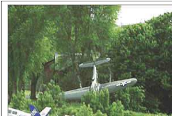
The day after a De Havilland Vampire "flicked-in" trailing in the wake of a De Havilland Sea-Vixen - the very next day the vintage P-63 Kingcobra "spun-in" from the top of a loop. (AAIB)
