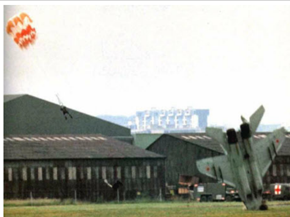
The close proximity of the ejected pilot to the aircraft impact point following a low-level ejection is clearly depicted in this MiG-29 crash at Paris Airshow in 1989. (Aviation & Week Space Technology)
