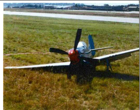
After exhausting all possible alternatives to extend the mechanically locked right main wheel, the only available option was to land with one main wheel retracted and one extended. (SAAF Museum)
