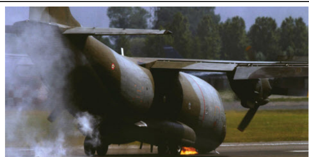
The sparks from the Italian Air Force's G-222 ignited a hydraulic fire which extinguished itself once the fluid had been exhausted. (Col A. Biasus, Brazilian Air Force)
