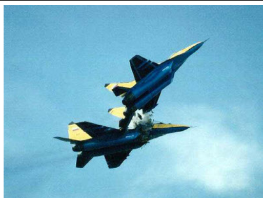
Moments after the collision, Tresvyatsky's aircraft "buckles" behind the cockpit and then explodes. Beschastnov's aircraft is seen pulling up and away with fuel spraying from the severed wingtip. (Aviation Week & Space Technology)
