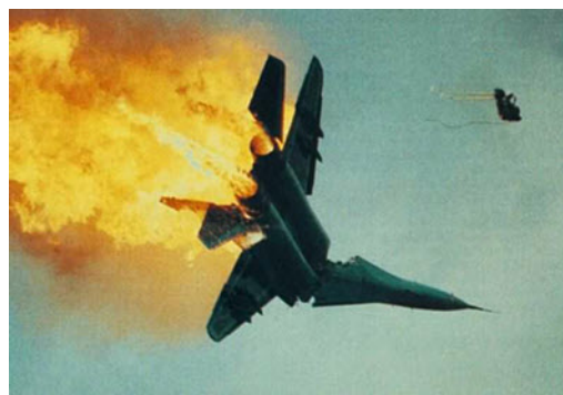
The blazing aircraft plummeting towards the ground. Tresvyatsky ejected while the aircraft was still erect, and the seat stabilizers have deployed. (Aviation Week & Space Technology)
