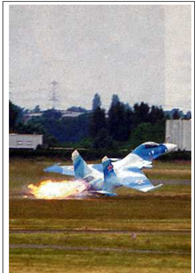
The twin-seat Sukhoi Su-30MK attempted to pull out of a descent that had included three 'high alpha' downline rolls using vectored thrust. ( Aviation Week and Space Technology )
