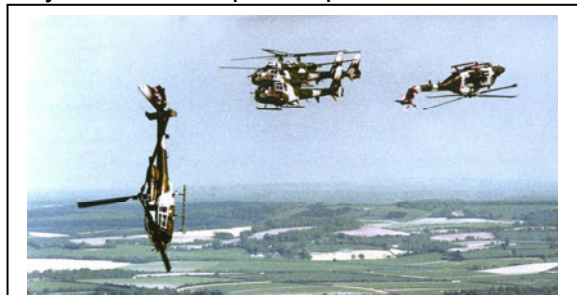
The Lynx, with its semi-rigid titanium rotor head, is capable of high manoeuvrability that not only enables the inimitable 'Backflip' to be flown, but also to combine its agility with the graceful four-ship Gazelle formation. (Blue Eagles)
