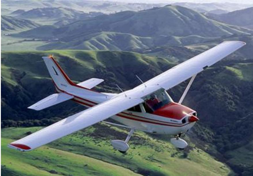
A 172 is spin resistant, the ailerons will work at the stall and during the recovery. One of the key design features that allow this is 'washout' which means that angle of attack of the outboard section of the wing is less than the inboard part of the wing. However whilst modern aircraft are docile, safe and easy to fly, all designs, old and new, produce lift in the same way; when the critical angle of attack for a wing is exceeded lift reduces, sometimes dramatically.
